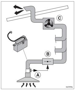
The potential free contact on the DSM 400 (a) can, for example, be used in a cooker hood with an external motor ...EXT, which is connected to a central ducting system.
